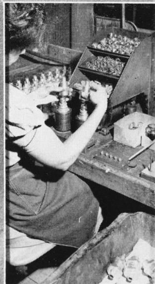
The girl at the left is assembling valves at Schrader for amphibious trucks that carry men and firepower from ships to shore and help to secure beach-heads. These tricky valves are arranged so that tire pressures can be controlled from the "duck's" cockpit.
